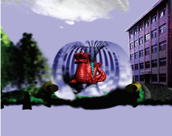
Figure 10. Sample image, after alpha blending the first 6100 slices of the 9900 total slices. The light source was located on the front-right side.
