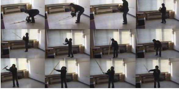
Figure 2: The calibration procedure starts with the user picking up the calibration pole and moving it around the motion tracking region. As is apparent from the sequence, the trajectory of the pole is free although the speed should be kept relatively slow to minimize interpolation errors.
