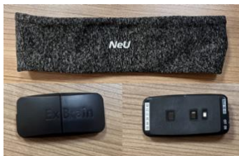
Figure 6: XB-01 brain sensor in a headband. A sensor must be placed in the upper area of the left eye.
