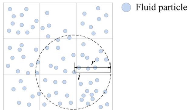
Figure 1. Neighborhood search with the uniform grid (2D): in the upper left, lower left, and upper right grids, there are no fluid particles within the influence radius  $r$  of the particle  $i$ .
