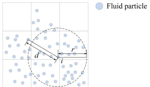
(b) Figure not displaying pruned fluid particles: Determine whether displayed fluid particles are within the influence radius  $r$  of the particle  $i$ . In a lower left grid, all registered particles are outside the influence radius  $r$ , but depending on a position of the particle  $i$  and AABB, they may not be pruned.
