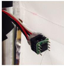
Figure 10: Sewing accelerometers onto nylon fabric.
