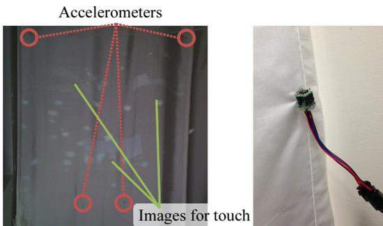
Figure 25: Sewing on accelerometers.
