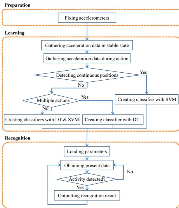
Figure 3: Flowchart for proposed method.
