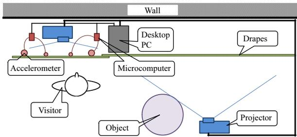
Figure 24: System structure of WPSS.
