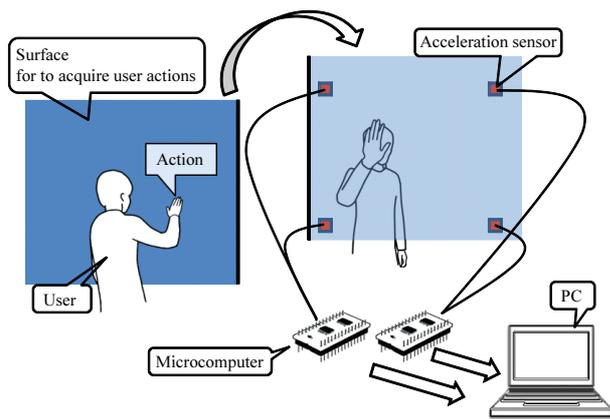
Figure 2: System structure.
